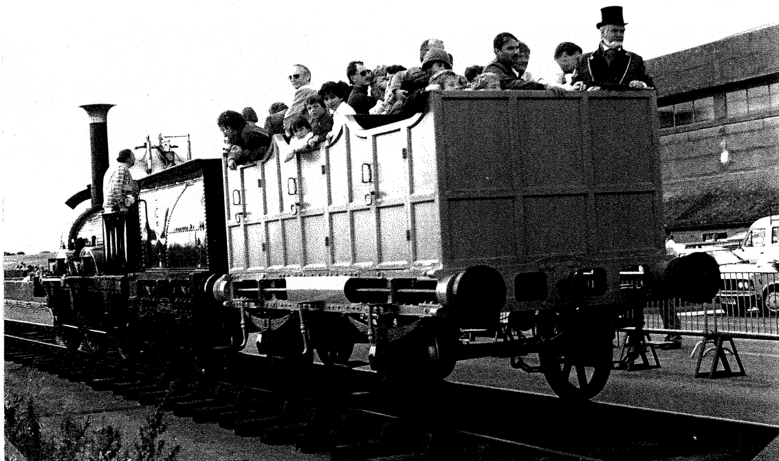
Photo 1. The 3rd class carriage coupled behind Lion at Wroughton in 1988. This was my first face to face meeting with Lion and some of the OLCO personnel. Far right in the topper is Charles Taylor-Nobbs, whilst far left is driver Jan Ford. Note the curved plate half way along the chassis, housing the square section buffer spring, connected to the buffers by the long buffer spindles. Thus all buffing loads are transmitted through the vehicle, rather than by it. Traction loads are treated in a similar fashion. Track is temporary.
