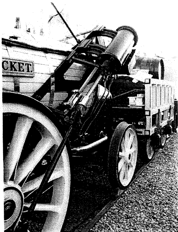
'Rocket', showing one of the copper circulating pipes connecting the firebox to the boiler. Note the angle of the cylinders, which exacerbated hammer blow on the rather weak track of the 1830s. Later Stephenson locomotives quickly adopted the horizontal (or almost horizontal) layout.
