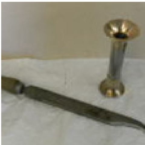
Photos 4 and 5. David Wilson's flared chimney, with profiled file and other tools.
